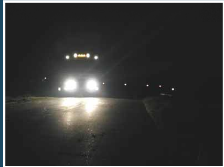
side marking lights (SML) (mandatory from 1996)
