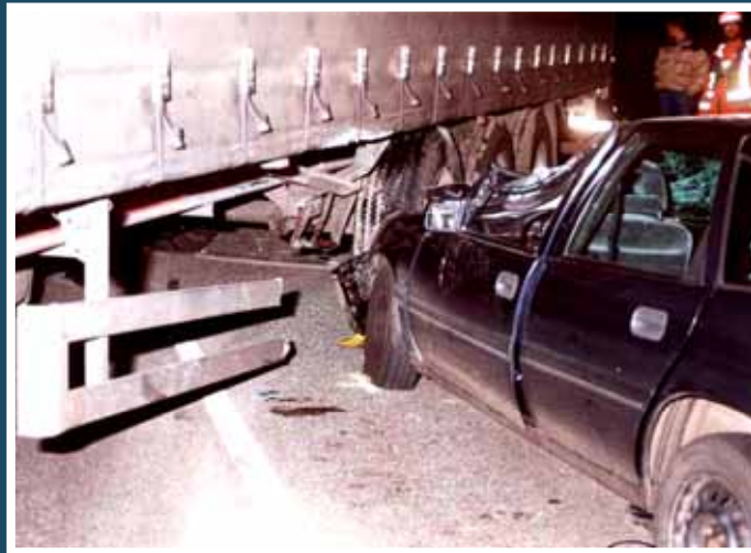
underrun (fatal for vehicle occupants)
